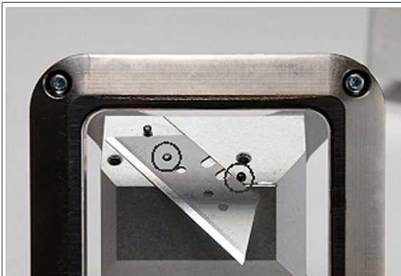
This picture shows how the knife blade is aligned using two guide pins beneath the blade clamping.
