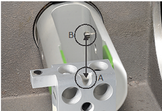
Turn the V-notch knife tool (A) correctly to fit the alignment pin (B).
