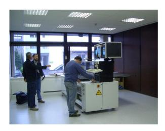
Flat mounting table, computer controlled for mounting flexo plates onto a milar for the corrugated industry
