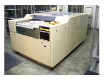
In-line platewasher in a self-contained design with integrated pre-dryer. Most modern technology.
