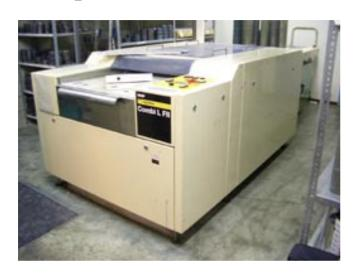
In-line platewasher in a self-contained design with integrated pre-dryer.
