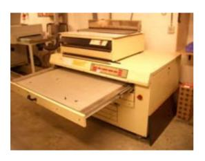
max. plate format 660 x 800 mm Width 1570 mm Depth 1200 mm Hight 880 mm Weight 450 kg Power
