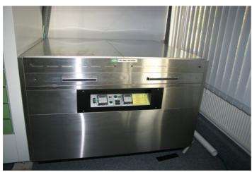
This Light-Finisher is designed to do the end-polymerisation of photopolymer plates. The tackines of plates will be drastically reduced. The complete polymerisation needs two steps. First the *finishing* with the built in UV-C bulbs, and second the *post exposure* with UV-A bulbs.
