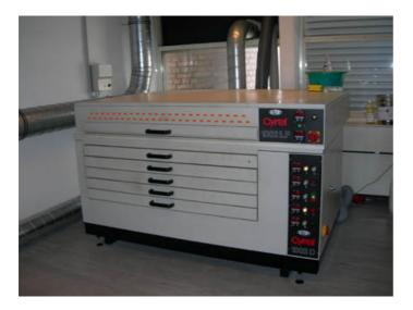
LIGHT-FINISHER For anti-tacking with UV-C + Post exposure with UV-A
