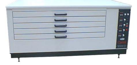
The finisher drawer is mounted on ball-slide and bears twenty-four UV-C tubes and twenty-five UV-A tubes.
