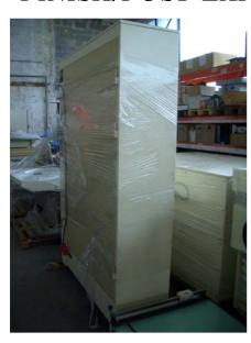
This Light-Finisher is designed to do the end-polymerisation of photopolymer plates.
