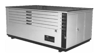
The 3000 D provides very even drying temperature and consistent airflow throughout the five separate drawers to provide excellent drying uniformity. A closed loop between the computer control board and the heating elements permits a carefully controlled temperature, preventing overheating of the plate base.
