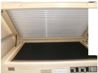
With this all-in-one-unit you are in the position to produce a plate size of 900 x 1200 mm.
