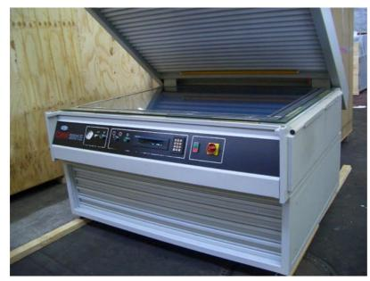
Exposure with glass plate for back and main exposure.
