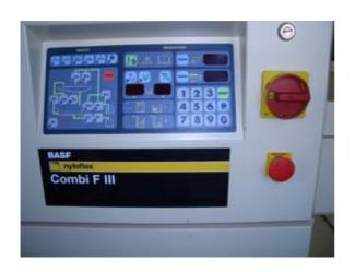
Year of manufacture 2001 90 x 120 cm Max. plate size Length 330 cm Width 170 cm Hight 120 cm Weight net 500 kg Weight gross 1400 kg Power requirements 5 kW
