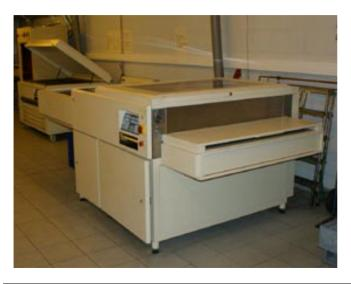
In-line platewasher in a self-contained design with integrated pre-dryer. Most modern technology.
