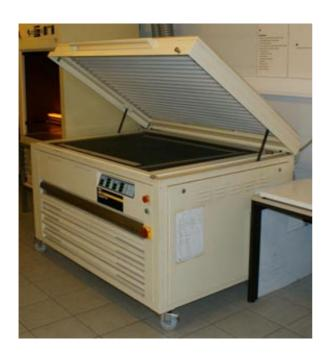
With this all-in-one-unit you are in the position to produce a plate size of 900 x 1200 mm.
