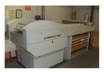
In-line platewasher in a self-contained design with integrated pre-dryer.
