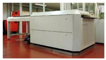
In-line platewasher in a selfcontained design with integrated pre-dryer.
