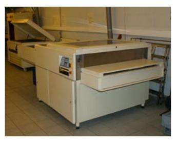
In-line platewasher in a self-contained design with integrated pre-dryer.
