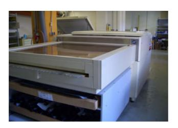
In-line platewasher in a self-contained design with integrated pre-dryer. Most modern technology.
