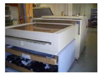
In-line platewasher in a self-contained design with integrated pre-dryer. Most modern technology.
